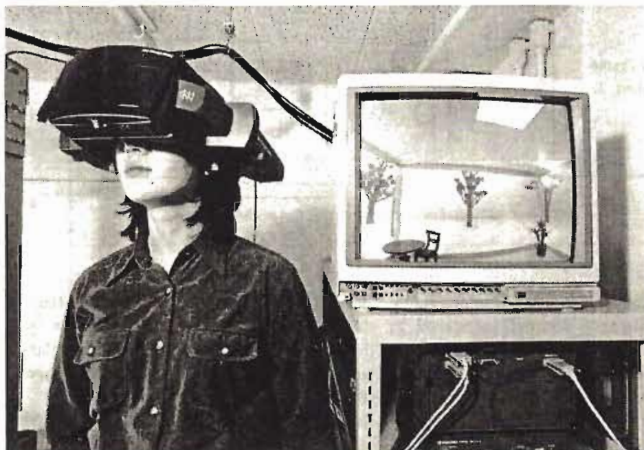
Figure 3. The subject wearing the HMD is looking around the interior space of the scale model. (The TV monitor shows the same visual image as the HMD)
